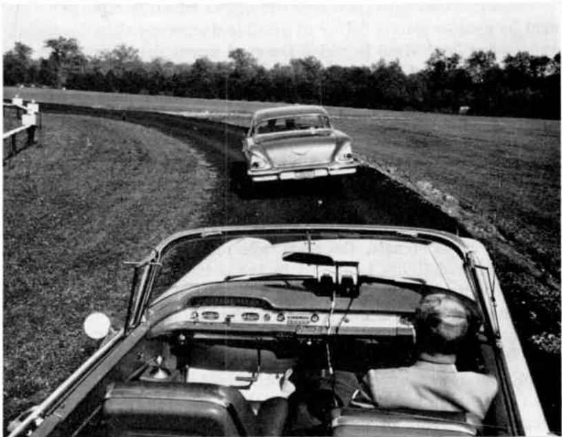
Fig. 13—"Equipped" car following a standard car on the RCA Laboratories test track. When the equipped vehicle is under manual control, steering, throttle control, and braking are performed with the "joy stick" control shown to the left of the driver's seat.
