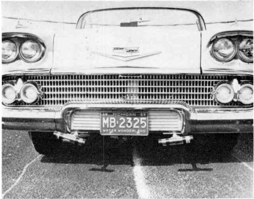
Fig. 1—Steering and spacing antennas on “equipped” car.
